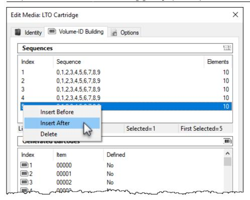
Any unwanted or unneeded ranges can be removed by right clicking the required index and selecting Delete.
