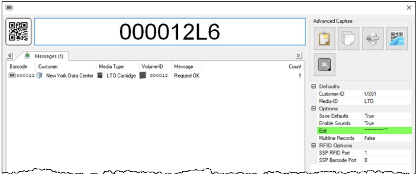
To remove a prefix from the barcode, inserting ^^~~~~~ into the Edit field will remove the first two characters from the barcode and keep the next 6 characters.
