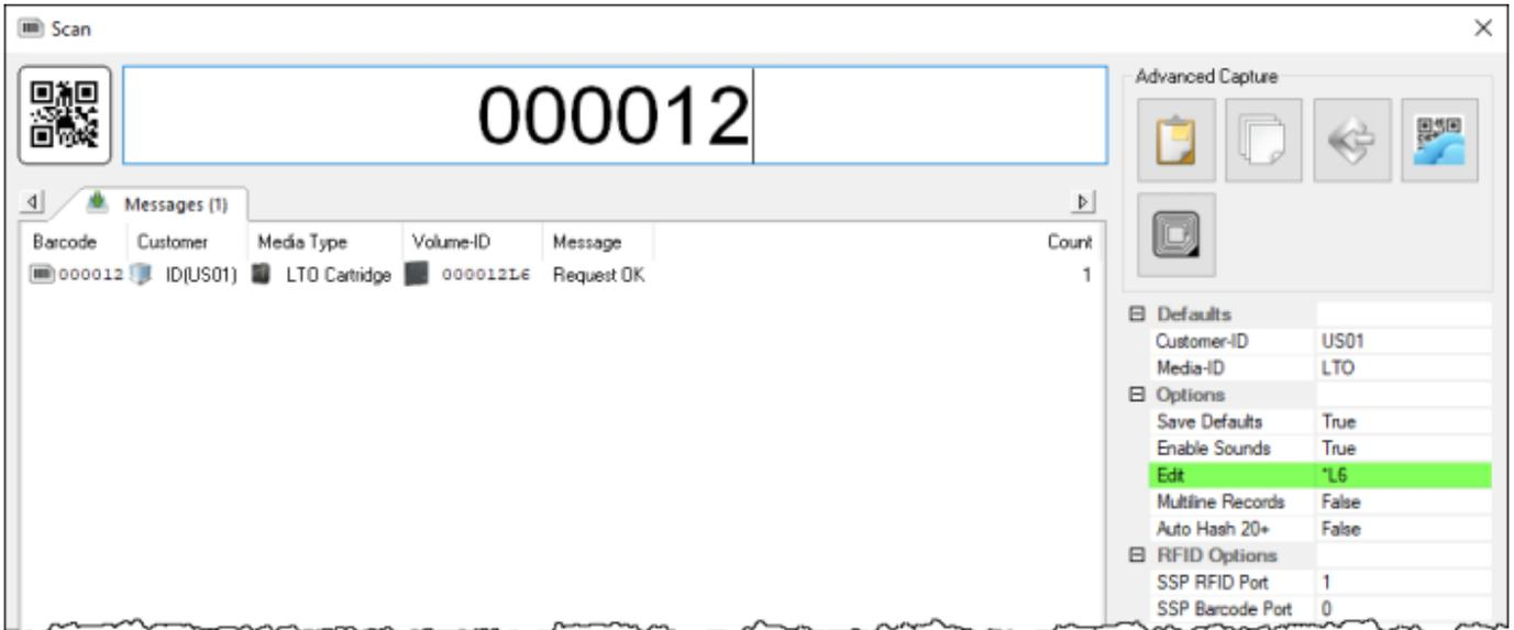
To add a prefix to the scanned barcode is achieved in the same way as adding a prefix except the prefix is added to the Edit field before the asterisk.
