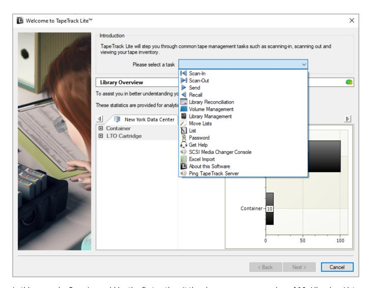
In this example, Scan-In would be the first option. It thus has a sequence number of 10. Likewise, List is the sixth option and thus has a sequence number of 60. To put a custom command between Recall and Manage, you could use the number "45" in the TMSSLite.cfg file to indicate that it is between the 4th and 5th option.
