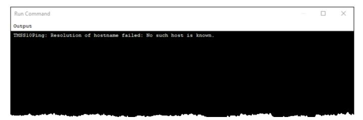
Contact your Server Administrator to ensure the correct IP address is entered into the Lite config file.
