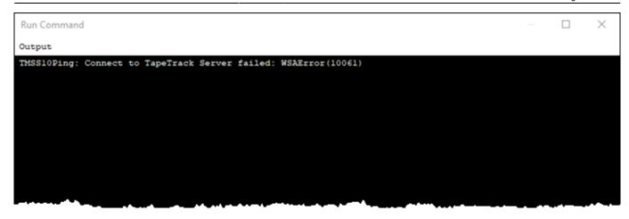
Contact your Server Administrator to ensure the TapeTrack Framework Server is running and your firewall is not blocking access to the Server ports.
