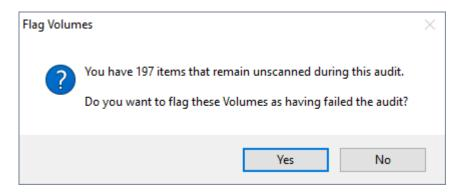
Updated flags will not be added to any volume/s with a current update lock applied to them and error window will be displayed as a result. The error window will display information on how many volumes were updated and which volumes are flagged with error status with an error explanation.
