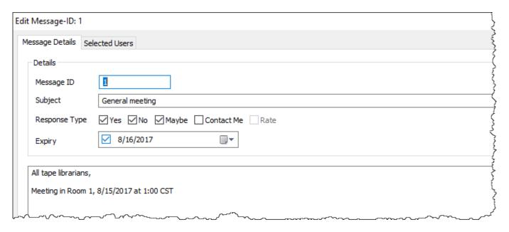
Users to receive the message can be chosen from the Selected Users tab. Select the user/s and press the spacebar to select or de-select the users that will receive the message. User responses (if any), along with the time and date, are also displayed
