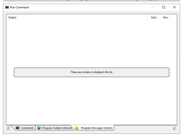
If the execution of the command encountered any errors they will be displayed in the Program Messages (stderr) tab.
