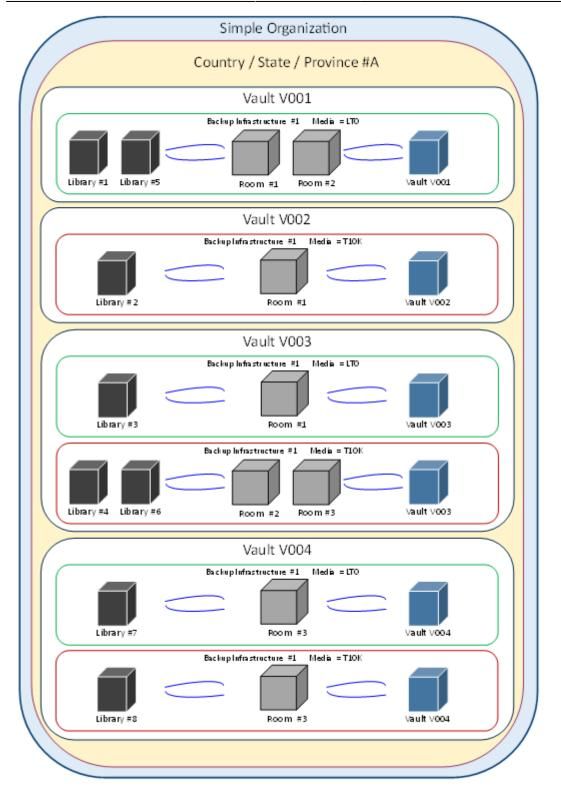
This could be translated into TapeTrack as a x4 Customer ID's representing the x4 off-site vaults, with LTO and T10K media that would still have a minimum of x3 Repository ID's per Media ID, as shown below.
