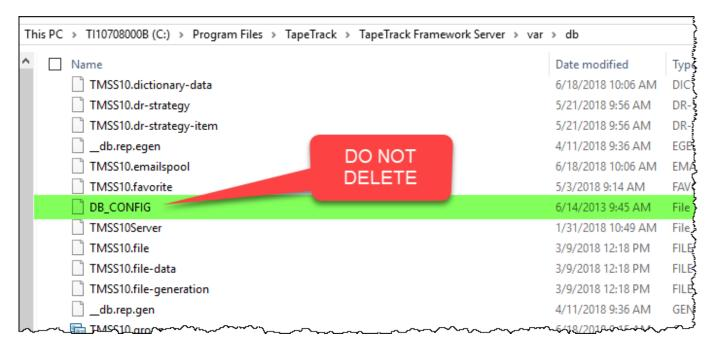
Edit the DB\_CONFIG file and remove the comments (#'s) starting from the line **rep-set-priority 0** to make the machine a Replicant.
