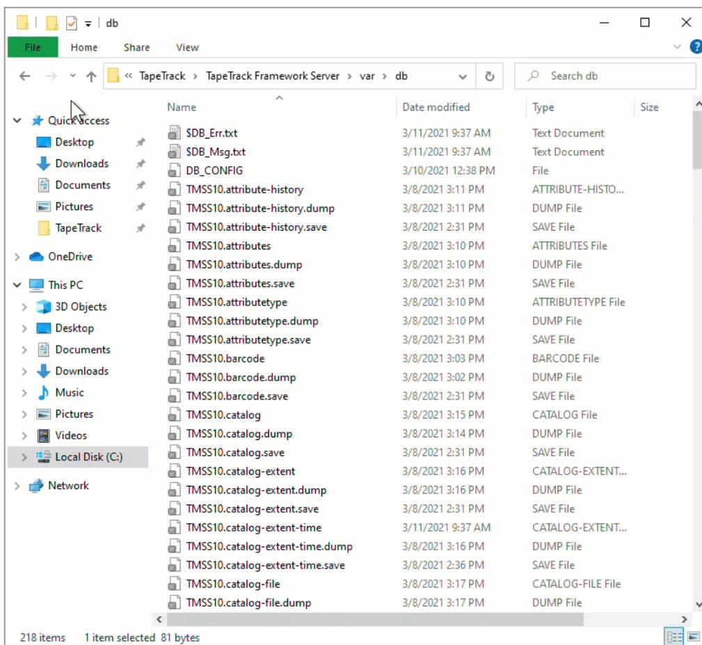
Edit the [DB\\_CONFIG](#) file and remove the comments (`#`'s) starting from the line **rep-set-priority 0** to make the machine a Replicant.
