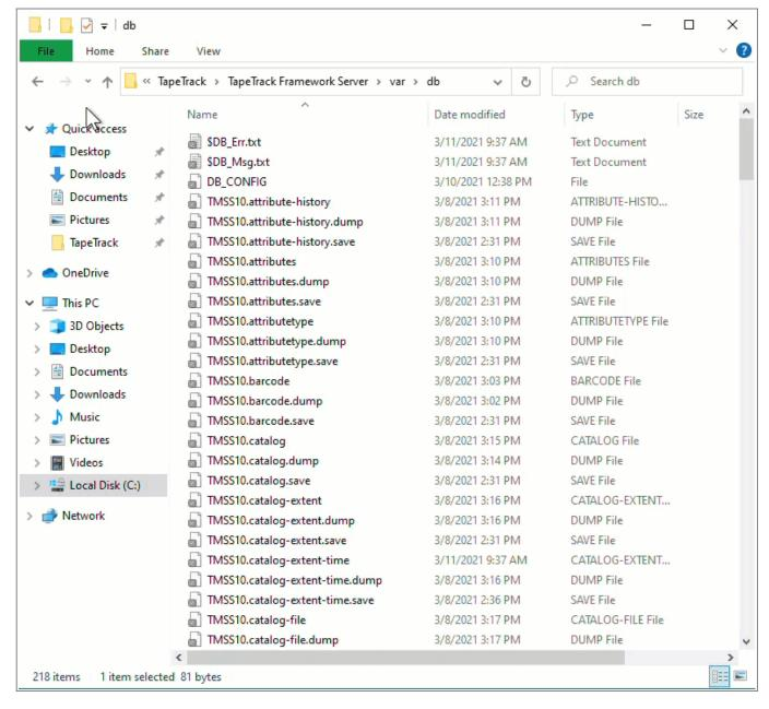
Edit the TapeTrack\TapeTrack Framework Server\DB\_CONFIG file and remove the comments (#'s) starting from the line **rep-set-priority 0** to make the machine a Replicant.
