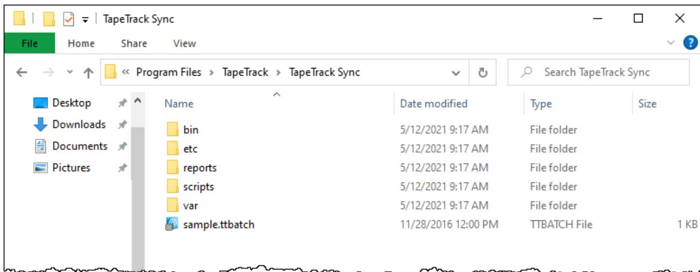
Conforming to this file layout for Sync inputs and outputs allows you to use relative file paths rather than absolute file paths. This increases the ease of reusing or moving the files between servers.
