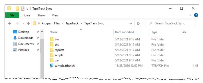
Conforming to this file layout for Sync inputs and outputs allows you to use relative file paths rather than absolute file paths. This increases the ease of reusing or moving the files between servers.
