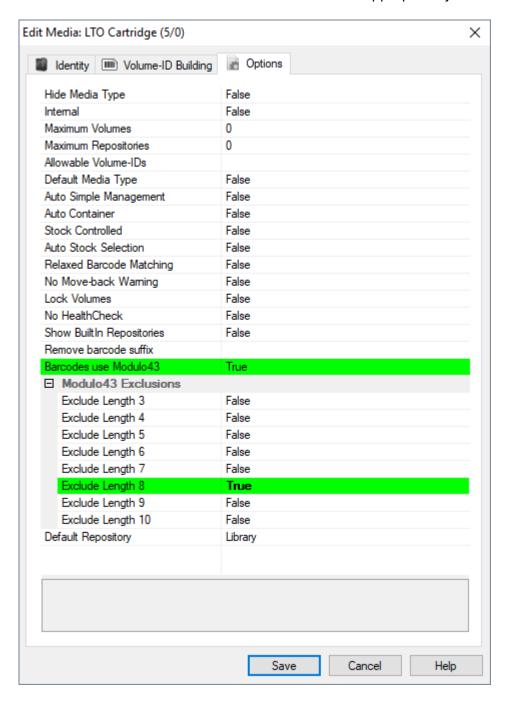
For example, Barcode **123456L6** will scan as **123456L6** without alteration, where as **22944L6B** will scan in as **22944L6**.
