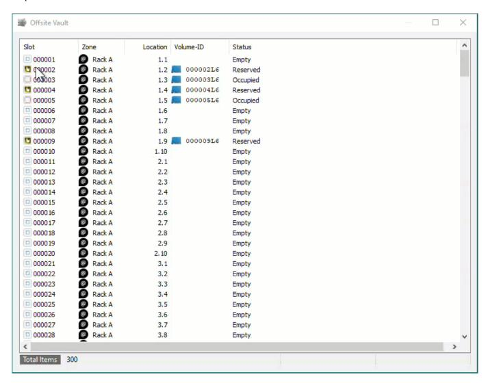
Intellislot will first attempt to find a range of Slots large enough to fit the Volumes in sequential Slots and, if a range can't be found, will then select other empty Slots to accommodate the required numbers.
