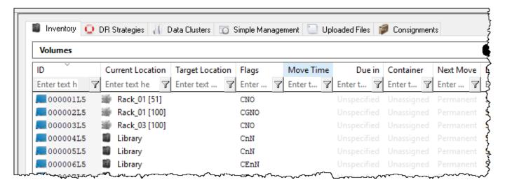
TapeTrack TapeMaster display with zone set to 10 slots per shelf. Display for volume 000001L5 shows in Zone Rack\_01, shelf 6, slot 1 (in the format **Zone\_ID [shelf#.slot#]**)
